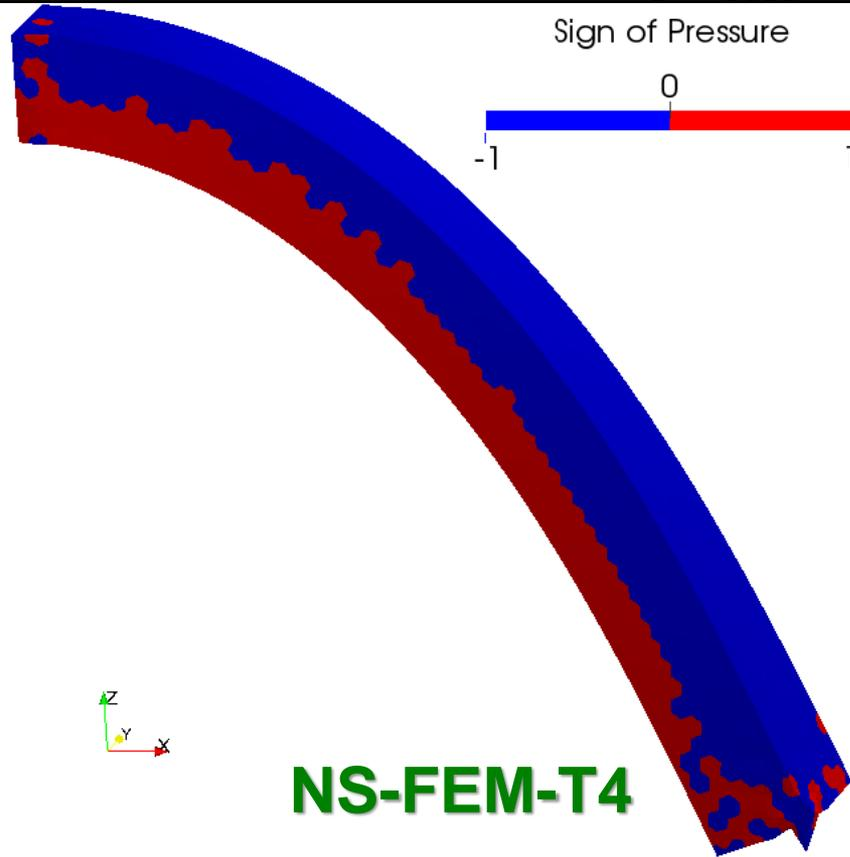
**NS-FEM** already suffers from minor pressure oscillation. The oscillation is magnified a little in Selective S-FEMs.
